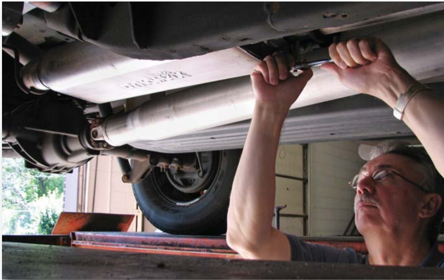
Nick Macaluso, engineering manager for performance products, installs an all-welded stainless-steel DynoMax performance muffler. DynoMax is Tenneco's premium performance-exhaust line.
