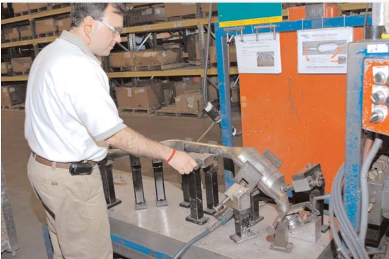
Ed Keshen, engineer/quality manager at the Harrisonburg facility, uses a fixture to check the fit on an OE application for Jaguar. Walker makes all its own fixtures and performs quality-control checks regularly. Many of its OE processes are used in aftermarket applications.
