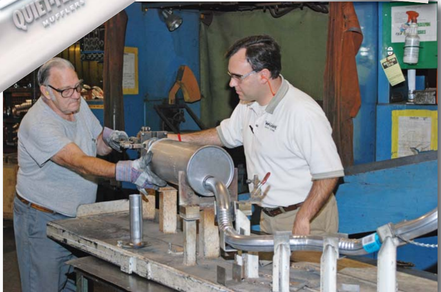
Veteran plant worker Roger Beale (left) and Ed Keshen, engineer/quality manager, check the fit of a 409-stainless-steel Quiet-FlowSS exhaust system.
